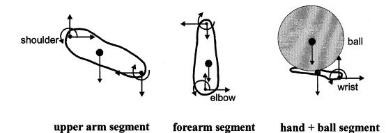
Figure 1 — Two-dimensional model, with muscle torque generators inserted at the shoulder, elbow, and wrist, used in simulating the wheelchair free throw. The origin for the system was located at the shoulder joint.
