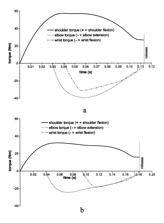
Figure 3 — Optimal torque histories from the three muscle torque generators using different starting positions. Fig 3a shows the torque histories produced by the model when starting from the position shown in Fig. 2a, while Fig. 3b shows the torque histories when starting from the position shown in Fig. 2b.
